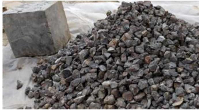
Figure 2: Recycled Concrete Aggregates (RCA)
